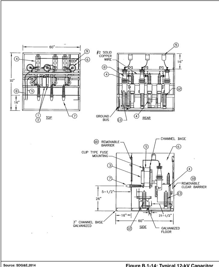
Figure B.1-14: Typical 12-kV Capacitor
